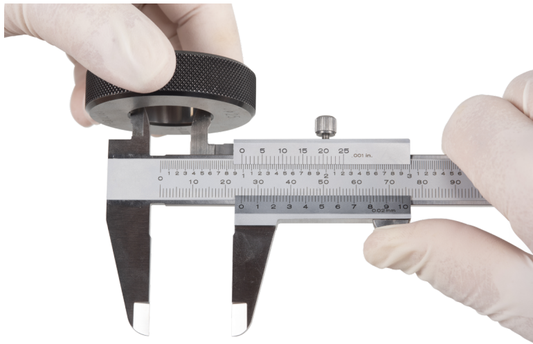
Figure 21: Measuring an inside diameter on a 25-mm master ring gage using a vernier caliper.
