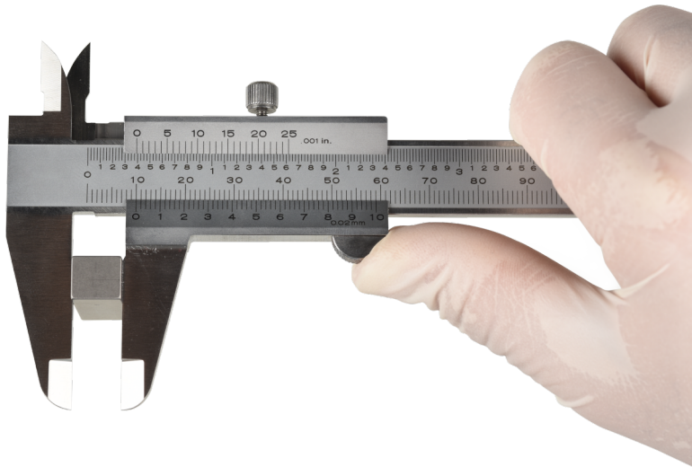
Figure 18: Checking the adjustment at the top of the jaws.
