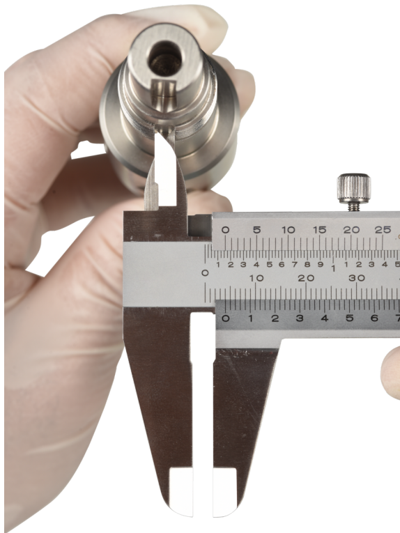
Figure 28: Measuring the width of a keyway ( L_3 ) on the pump shaft using a vernier caliper.
