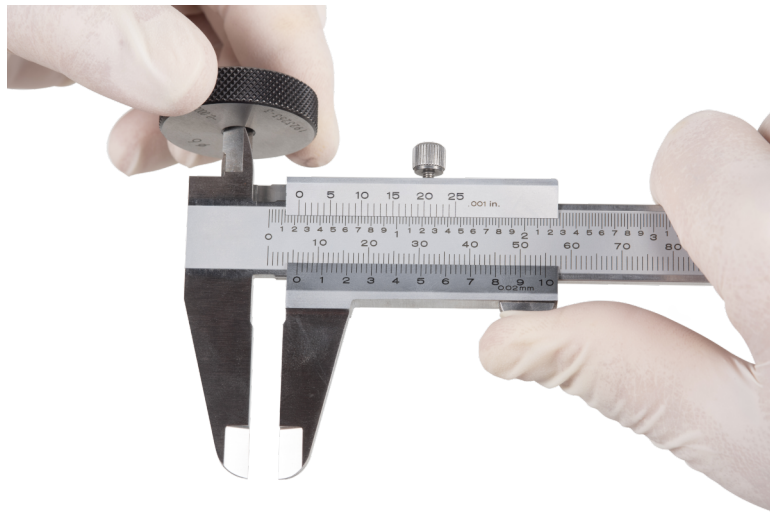
Figure 23: Measuring an inside diameter on a 6-mm master ring gage using a vernier caliper.
