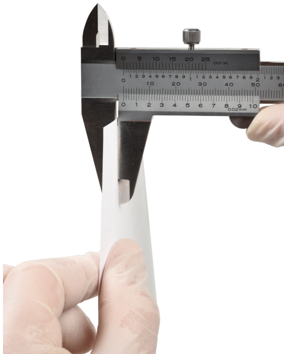
Figure 16: Cleaning up the measuring surfaces on a vernier caliper.
