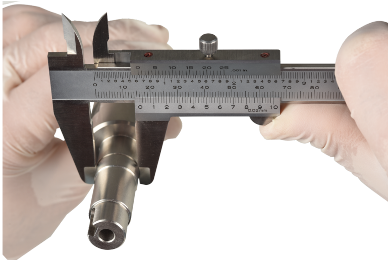
Figure 27: Measuring outside diameter F on the pump shaft using a vernier caliper.
